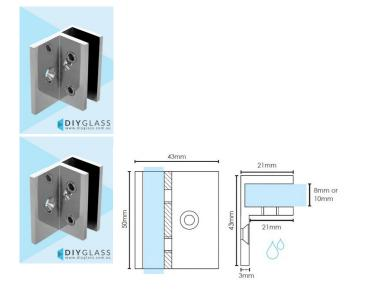
Used to fix Hinge and Return/Fixed panels to the wall in a shower screen.
