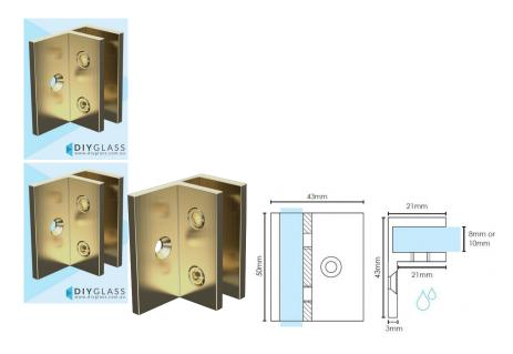
Used to fix Hinge and Return/Fixed panels to the wall in a shower screen.
