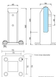
Stainless Steel Square Base Plate Spigot plus a thermoplastic non-conductive insulating sleeve that fits over the top.
