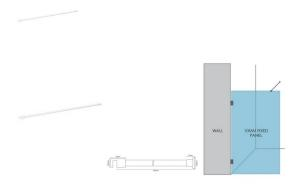
Used to stiffen and brace a Return/Fixed panel by connecting it to the adjacent wall.
