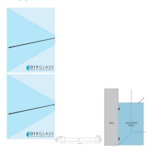
Used to stiffen and brace a Return/Fixed panel by connecting it to the adjacent wall.
