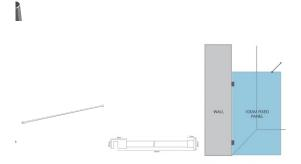
Used to stiffen and brace a Return/Fixed panel by connecting it to the adjacent wall.
