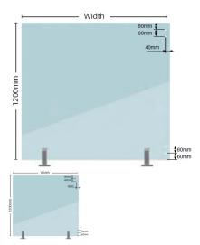
Glass Gate Spring Hinge Panel. Used to swing a glass gate off.
