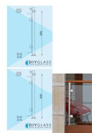
50x50 Square Glass Clamp End Post for Timber Rail •Position: End •Use: Glass Balustrade •Material: 50x50 Satin Finish Stainless Steel •Height: 970mm •Grade: 316 Marine Grade Stainless •Base: 4 Hole Square Flange •Top: 2 Hole Rectangle Flange •Glass: Install with 850mm Glass Panels •Handrail: Install with Timber Handrail
