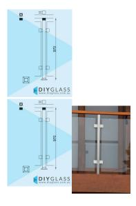
•Position: Centre •Use: Glass Balustrade •Material: 50x50 Satin Finish Stainless Steel •Height: 970mm •Grade: 316 Marine Grade Stainless •Base: 4 Hole Square Flange •Top: 2 Hole Rectangle Flange •Glass: Install with 850mm Glass Panels •Handrail: Install with Timber Handrail
