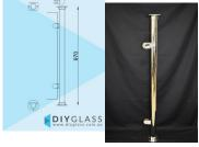
2" Round Glass Clamp End Post for Timber Rail •Position: End •Use: Glass Balustrade •Material: 2" Mirror Finish Tube •Height: 970mm •Grade: 316 Marine Grade Stainless •Base: 3 Hole Round Flange •Top: 2 Hole Oblong Flange •Glass: Install with 850mm Glass Panels •Handrail: Install with Timber Handrail
