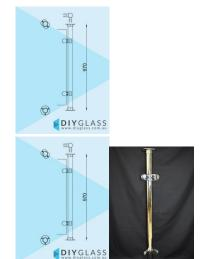
2" Round Glass Clamp Corner Post for Timber Rail •Position: Corner •Use: Glass Balustrade •Material: 2" Mirror Finish Tube •Height: 970mm •Grade: 316 Marine Grade Stainless •Base: 3 Hole Round Flange •Top: 2 Hole Oblong Flange •Glass: Install with 850mm Glass Panels •Handrail: Install with Timber Handrail
