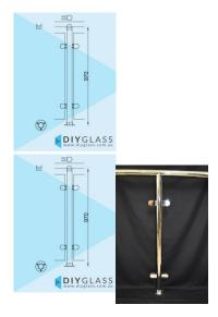
2" Round Glass Clamp Centre Post for Stainless Top Rail •Position: Centre •Use: Glass Balustrade •Material: 2" Mirror Finish Tube •Height: 970mm •Grade: 316 Marine Grade Stainless •Base: 4 Hole Square Flange •Top: Perpendicular Joiner •Glass: Install with 850mm Glass Panels •Handrail: Install with 2 Inch Round Stainless Top Rail The perpendicular joiner is Tek screwed to the underside of the rail then glued and riveted into the top of the post.
