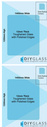
1400 x 1200mm Glass Pool Fence or Balustrade Panel
