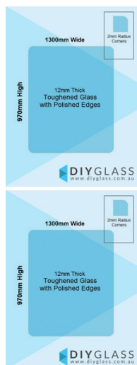
1300 x 970 Toughened Glass Balustrade Panel
