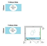
Glass Brace panel used to Connect the hinge panel to a return panel about the door.
